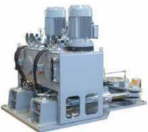
Factory Acceptance Test of the electronic synchronized steering gear type DDS 12000-35x2 which is manufactured for the Logistic Supply Vessel built for Turkish Navy (LSV) is accomplished with the attendance of authorities from Turkish Navy, Turkish Lloyd and Selah Shipyard. System is composed of 2 pieces 120 kN.m steering gears. Steering gears are mechanically and hydraulically independent from each other and electronically synchronized.
